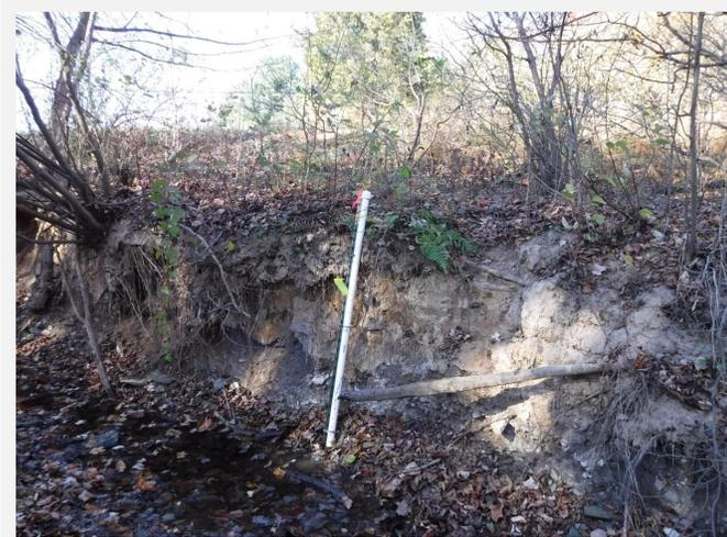
*2" x 6' PVC with pressure transducer for stage height analysis*
