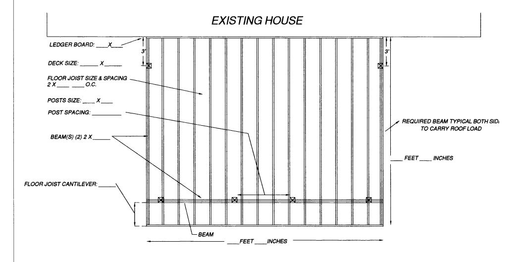
TYPICAL DECK FLOOR FRAMING FOR A RETURN GABLE ROOF ABOVE
