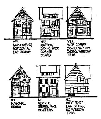
Replacing sound or repairable historic siding material is never recommended. However, if the historic material cannot be repaired because of the extent of deterioration or damage, then it will be necessary to replace it. The preferred treatment is always replacement in kind, that is, with the same material. A substitute siding material, such as aluminum or vinyl, should only be
