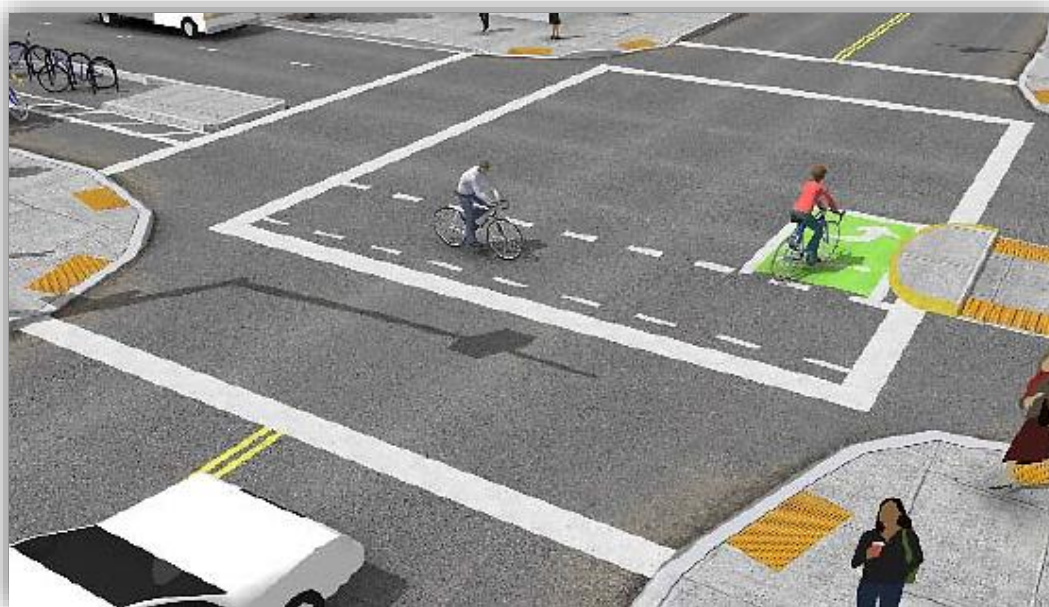
Figure 7-16: Two-Stage Turn Queue Boxes, NACTO p. 150
