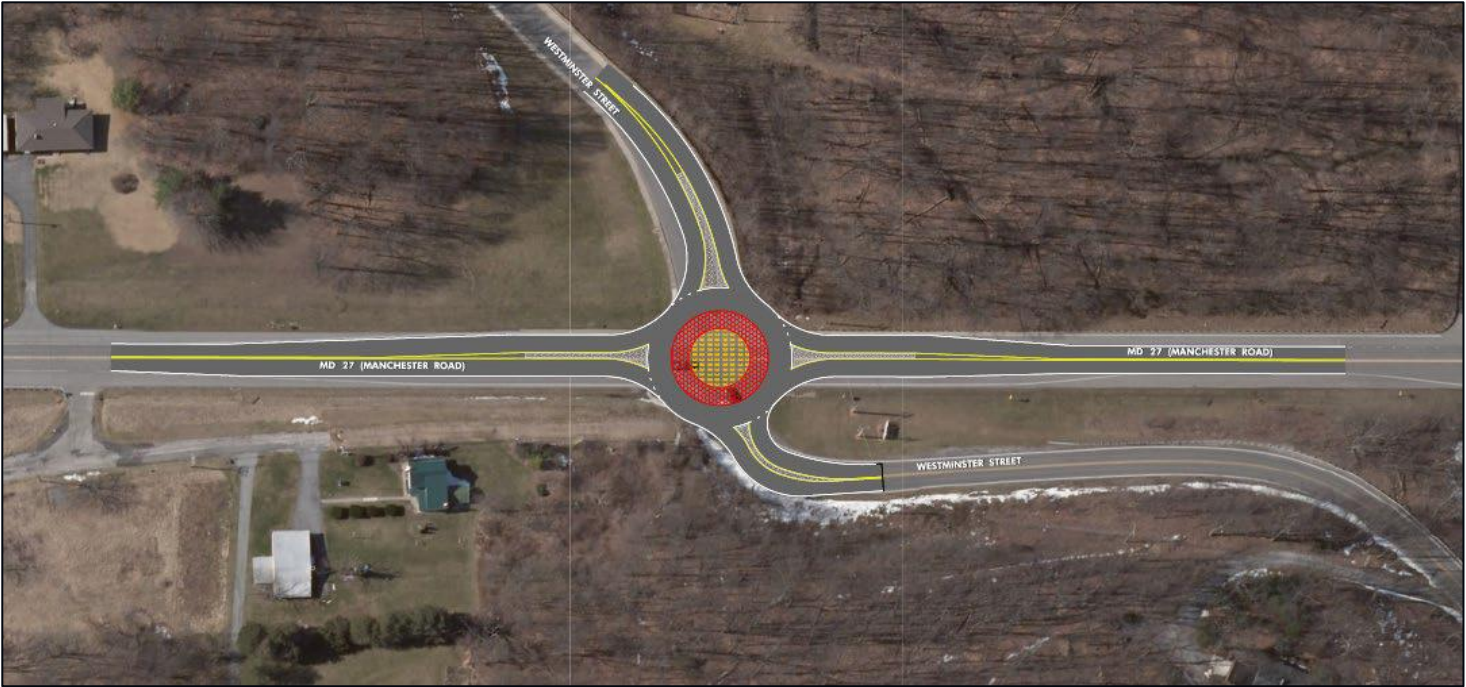
Figure 5.31 MD 27/Westminster Street Roundabout Concept
