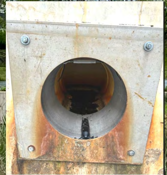
Orifice w/ U20L HOB0 Pressure Sensor
